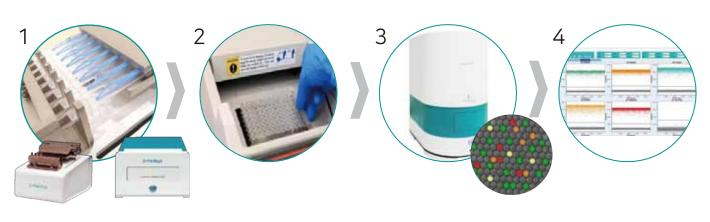
Load and partition Seal Thermal cycle Detect & Quantify
